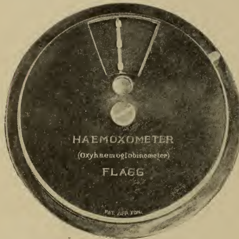
FIG. 58.—The Hæmoxometer (oxyhæmoglobinometer,) an instrument for the clinical measurement of cyanosis (oxygen unsaturation).
